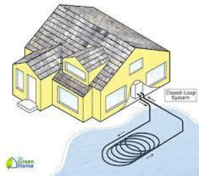
Fig. 35: Types and principles of heat pump (ground; water; air)
