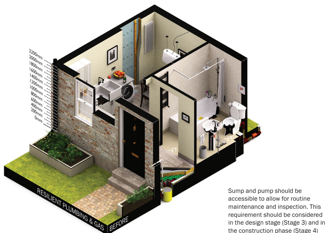
Figure 17.2 Sump and pump installed in a property (courtesy The Environmental Design Studio)
