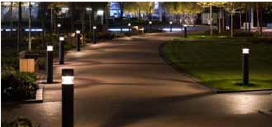
Fig. 32: Example of bollard lighting for pedestrians
